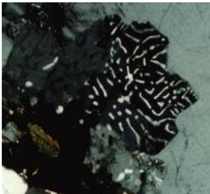
Fig. 7. Quartz vermicules of intermediate size in myrmekite (center) enclosed in K-feldspar (light gray). Coexisting biotite occurs enclosed in plagioclase (black).
